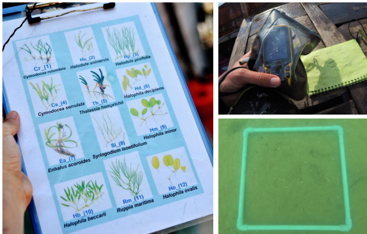
Figure 5. Seagrass survey equipment used. Left: dive slate with seagrass identification guide; Top Right: a handheld Garmin GPS device and a notepad for recording seagrass data and survey locations; Bottom Right: a 0.5m 2 quadrat distributed twice at each survey point, the area within the quadrat was measured for seagrass species, percentage cover and substrate type.
